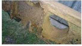
Strip down to chassis fairly straight forward, had to remove tank (rear fill) first before undoing rear cross member to body bolts which was a pain so captive nuts needed on rebuild to allow tank to be fitted before body (as it turned out the tank I took off was weeping slightly so new tank ordered)
