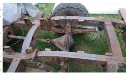
Lesson - most of the underside bolts and nuts where corroded (the bolt ends sticking out from the nut) so either sheared, had to be cut off with grinder with a couple having to use a nut splitter (well recommended to have these I have a draper set of 3 sizes). Going to underseal all the bolts/nuts.
