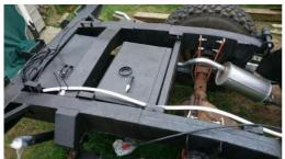
coverage and dries quickly ready for second coat in under an hour, and then used their no prep aerosol wax on the inside parts (comes with a long tube with a 'fan' spray head on the end). Made one mistake with the CIO as used white spirits to clean/store the brush but did not clean it thoroughly enough that it has contaminated the paint but my fault (can't fault buzzweld as the guy spotted this on my Facebook posts and let me know).
