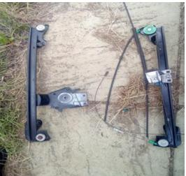
capture points in the door for placing and window adjustments O/s/r with motor only 3 bolts to loosen
