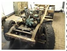
threaded holes were checked for any excess galvanic deposits and retapped where necessary. The chassis was then painted with two coats of black chassis paint. All coats were applied where possible by roller which gives a much more even coat than a brush.
