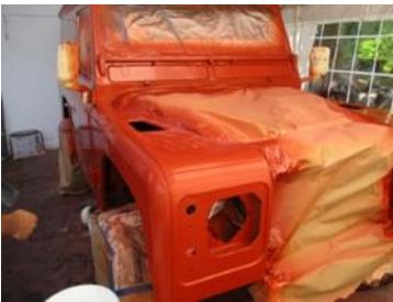
So now we are in April, Phoenix wasn't in great shape as he needed a lot of panel fettling with aluminium fillers and special zinc primer to hold the corrosion. Once the major dents were pulled out and re-riveted, the 3 coats of filler primer was applied wet and drying between all coats, the base of the orange mid part of the orange and then the final drop coat of the orange was applied and then 3 lacquers... yes 3!
